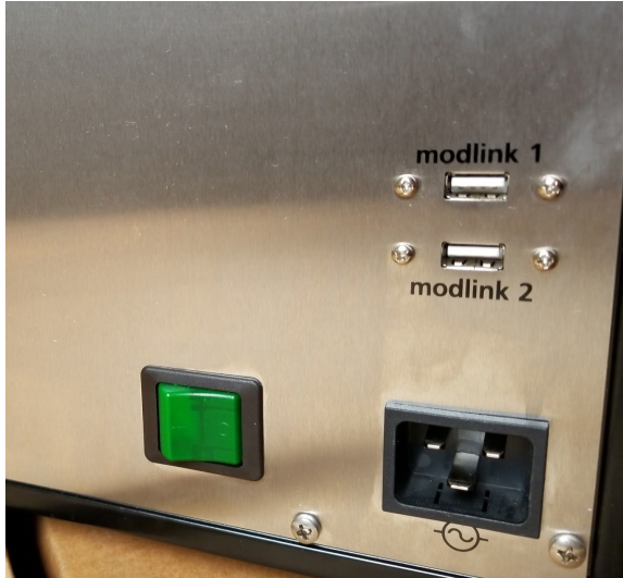
Rear Switch - Mains Power
