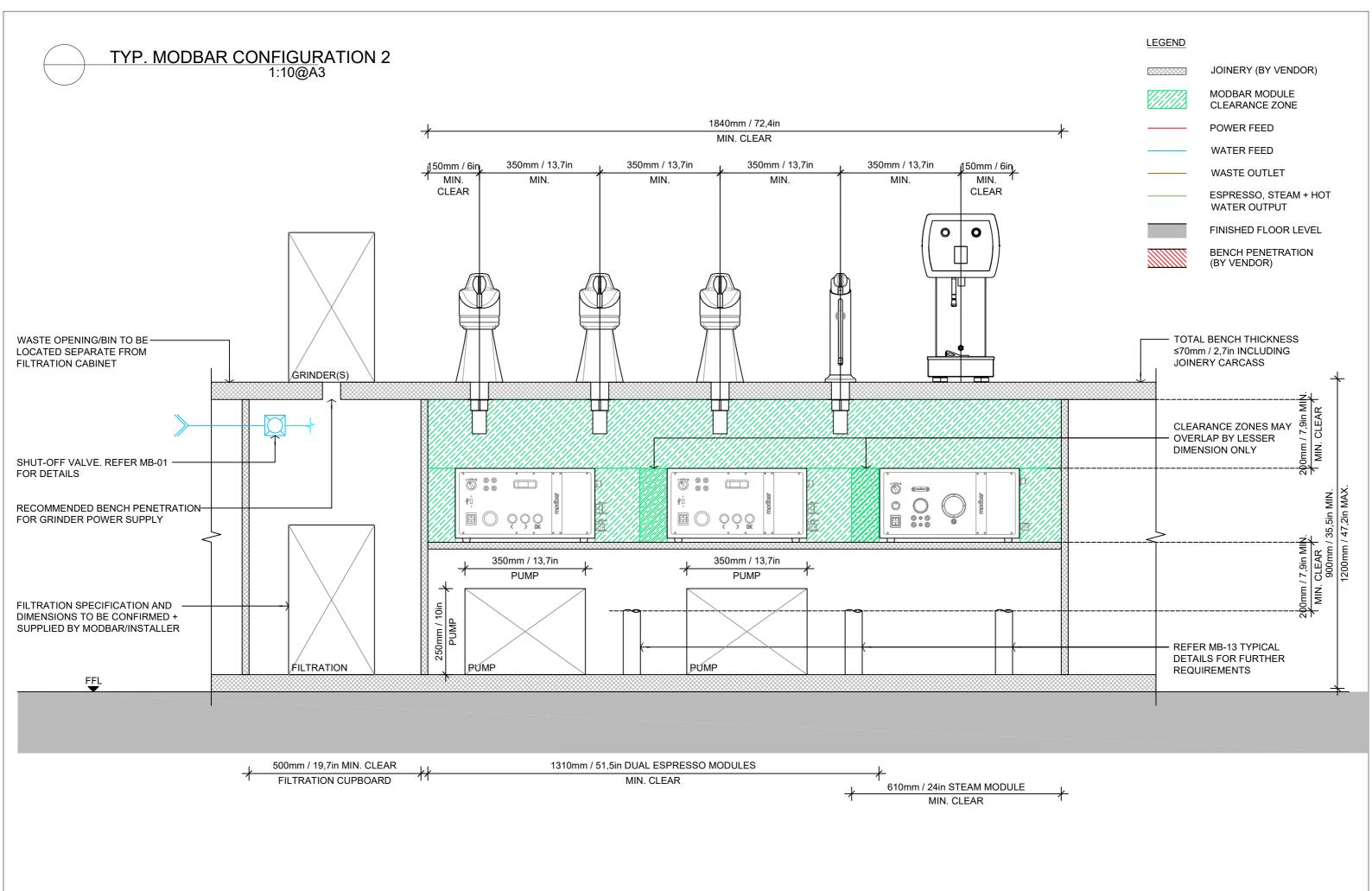
UNLESS NOTED OTHERWISE, ALL DIMENSIONS ARE IN MILLIMETERS. ANY ERRORS, DISCREPANCIES, OMISSIONS IN THE DRAWINGS, NOTATIONS OR DIMENSIONS SHALL BE IMMEDIATELY REPORTED TO MODBAR FOR CLARIFICATION PRIOR TO WORKS COMMENCING. DO NOT SCALE FROM DRAWINGS.
