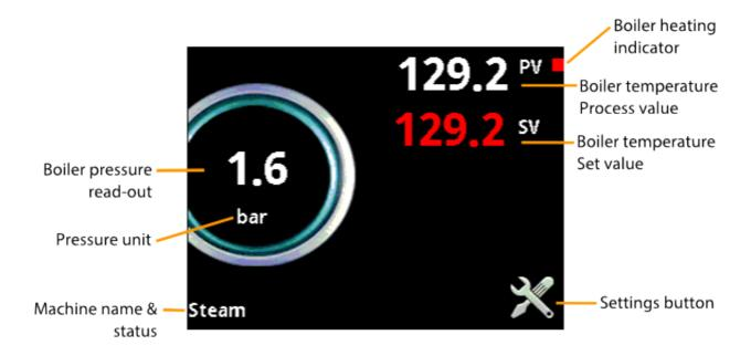
**Boiler heating indicator:** The red square indicates that the boiler is being commanded to heat. It is normal for this to flash on and off during regular operation.
