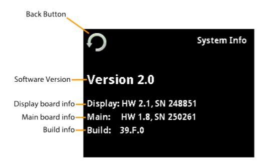
**Software Version:** This field displays the current software version loaded on the machine.
