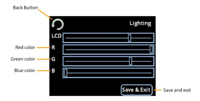
**LCD backlight:** Use this slider to control the brightness of the touch screen display.
